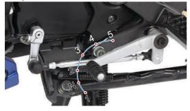
To shift the transmission from neutral to first gear, push the gear shift lever down.
