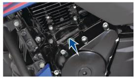
Engine serial number is engraved on the left side crankcase assembly near cylinder block as shown in the above figure.
