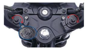
TVS Apache RTR 200 4V front suspension level can be adjusted as per your convenience. Adjust the suspension level as per the load or road conditions.
